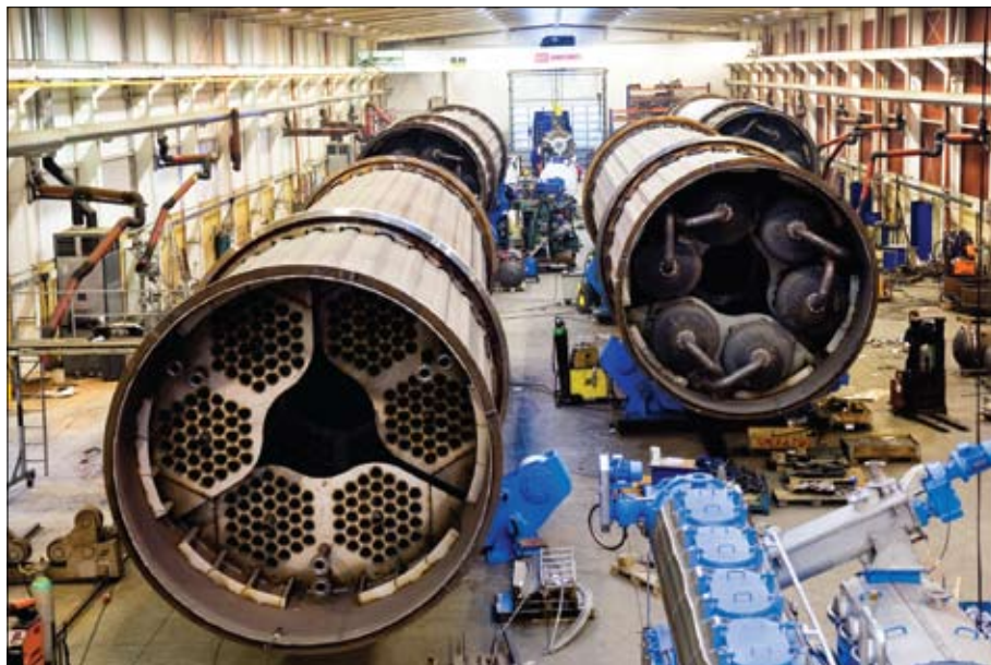
From the production of four RTD dryers for mechanical dewatering of stillage at Lantmännen Agroetanol AB in Sweden. Each dryer represents a heating surface of 1900 m 2 . Altogether, these four drying machines evaporate 40.000 litres of water/hour.
