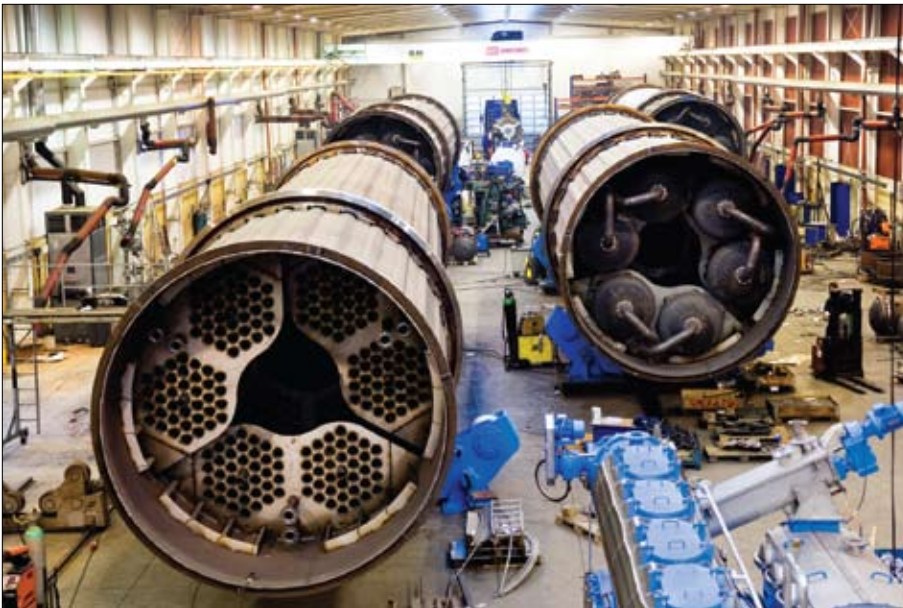
From the production of four RTD dryers for mechanical dewatering of stillage at Lantmännen Agroetanol AB in Sweden. Each dryer represents a heating surface of 1900 m 2 . Altogether, these four drying machines evaporate 9080 gallons of water/hour.
